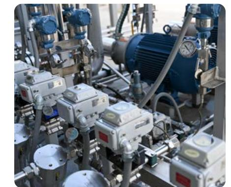
**Consolidated auxiliary skid** cuts installation hours, simplifies maintenance with a gearbox-less water pump, and facilitates winterization using a standard enclosure.
